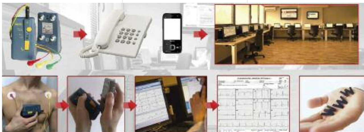
Figure 1. A complete 12-lead electrocardiogram may be recorded anywhere in a couple of minutes by the CardioVox P12 pocket recorder. After telephone coupling (mobile or other), the electrocardiogram is sent to the telecardiology hub, where a cardiologist available 24/7 analyses the data on his/her computer screen and reports back on the electrocardiogram. The electrocardiogram and the report may be sent back by telephone or internet and visualised on a smart-phone, iPad or computer screen, or printed off.
